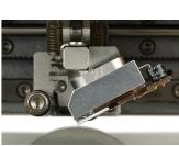
**AutoAlign**, our unique (patent pending) head control technology, simplifies installation. At the touch of a button, the print head automatically aligns to the optimum position, without the need for shims or tools. There is also no need supply or connect compressed air.
