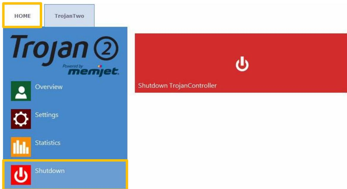
6. After shutting down the machine, turn off the power switch at the back of the machine to cut down power from the Power Supply Units.
