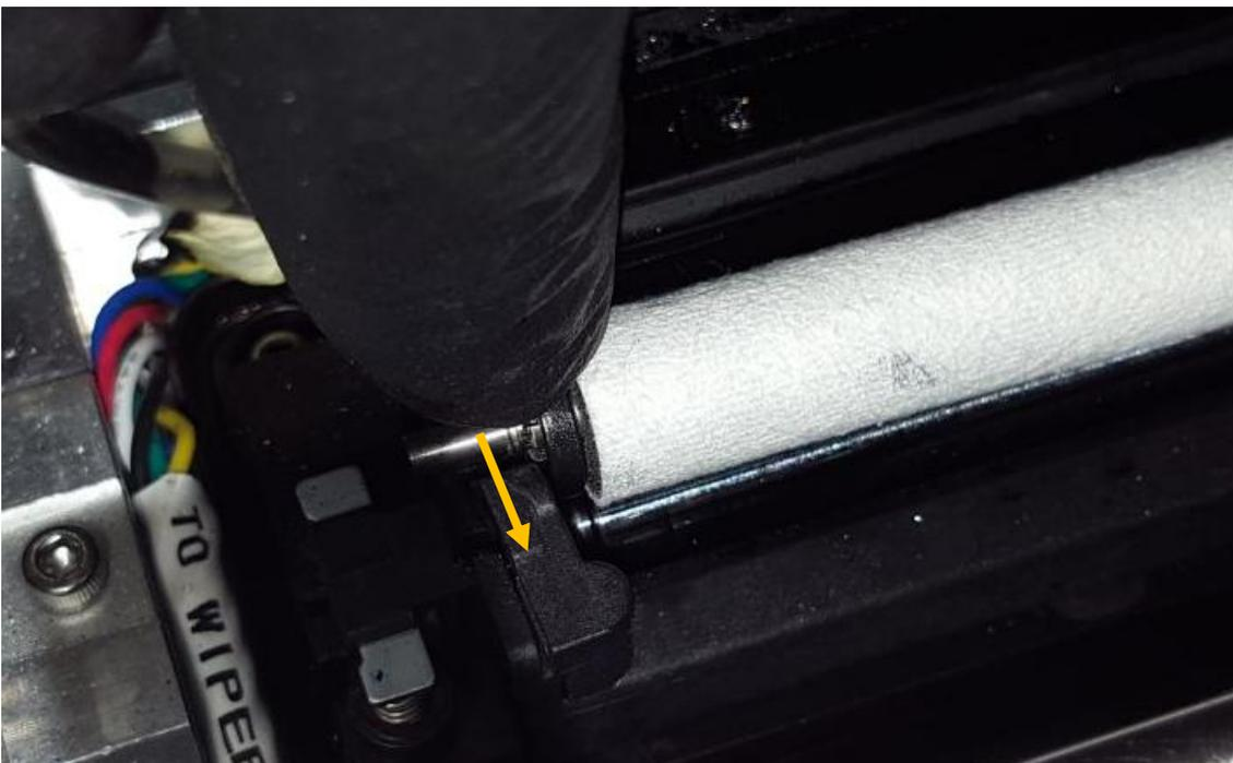
*Push the axis of the micro fibre roller under the plastic latch until it clicks onto the right place.*
