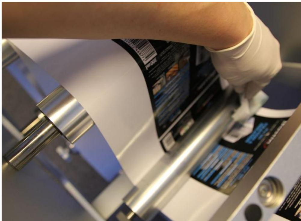
*Wipe each roller using a lint-free cloth and distilled water.*
