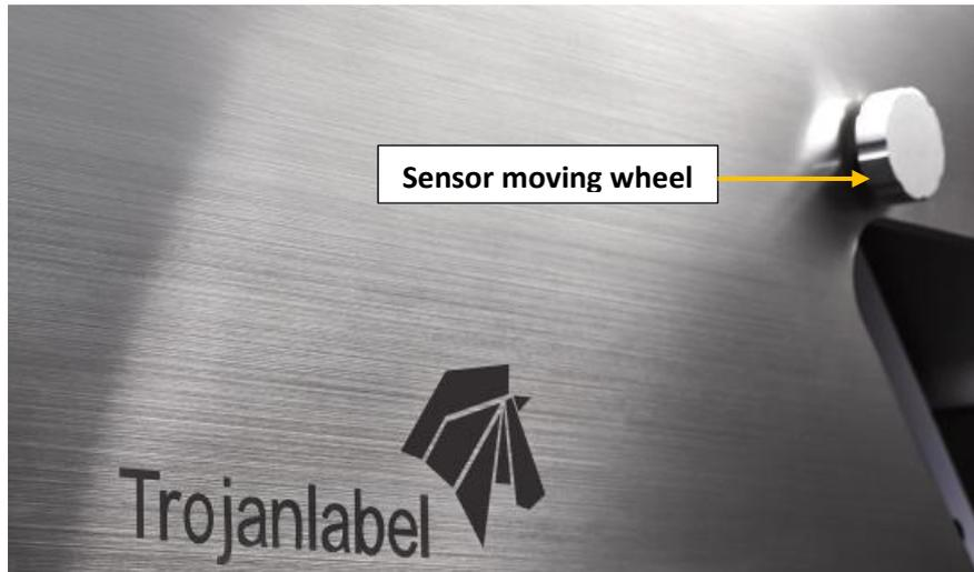
2. Move the sensor above a blackmark exactly where the sensor beam is to be able to teach the sensor to recognize the density of the registration mark.
