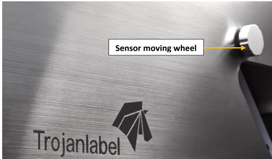
2. Move the sensor above a label gap exactly or peel off a label from the liner temporarily where the sensor beam is to be able to teach the sensor to recognize the label gap.
