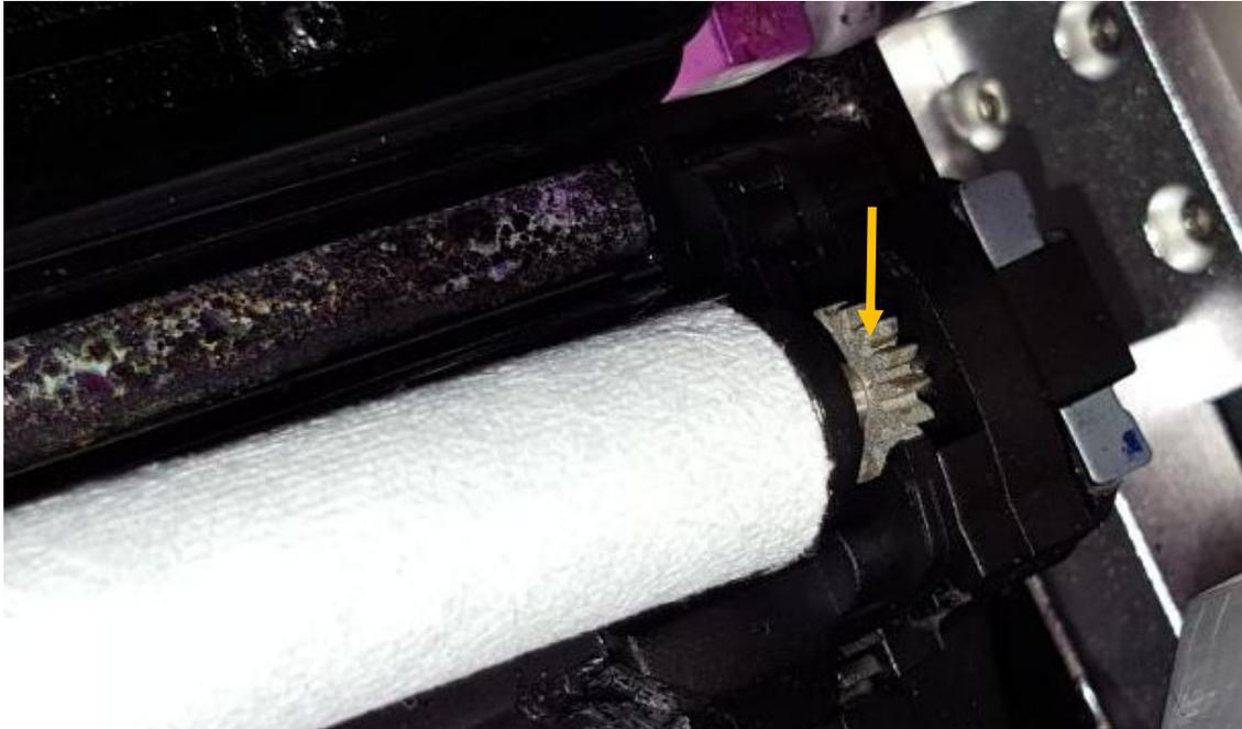
*Fit the gear on the right end of the micro fibre roller onto the proper place from above. The gear has to fit to the gear of the wiper motor.*
