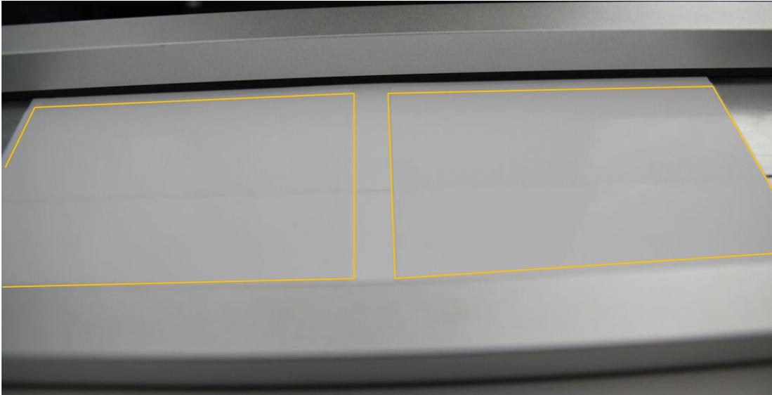
*Tape applied on upper side of label material.*
