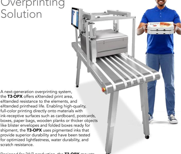
Designed for 24/7 production, the **T3-OPX** mounts on host systems with runs up to 18 ips; automatically adjusting for variances in speed, timing, and spacing. With brilliant automized height calibration and stable, high-quality production, the T3-OPX delivers ROI to businesses by easily expanding products and services to attract new and current customers with private labeling for seasonal or promotional events.
