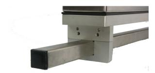
The 32mm diameter brackets allow 10mm of perpendicular movement which is useful for fine adjustment of Traverser position. Slots are provided in the brackets to accept locking rings (Domino Part No 5-0161129) these give additional anti-rotation support.
